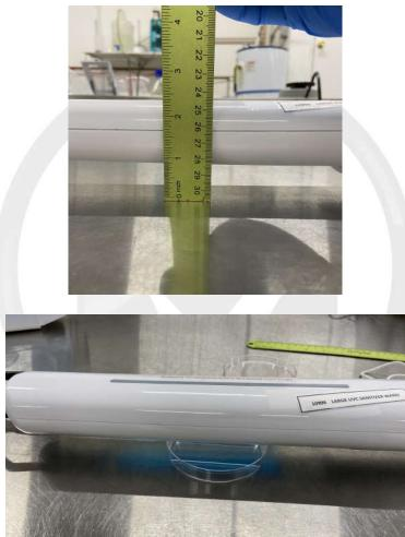
Note: (Top) Picture shows study setup with Item 10996. (Bottom) Picture shows carriers were placed directly underneath UVC lamp during the study for the entirety of the contact time.
